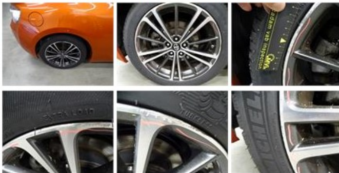
Alloy rim F L polished, Scratch(es), LI - Repair and paint (complete) 95,00
