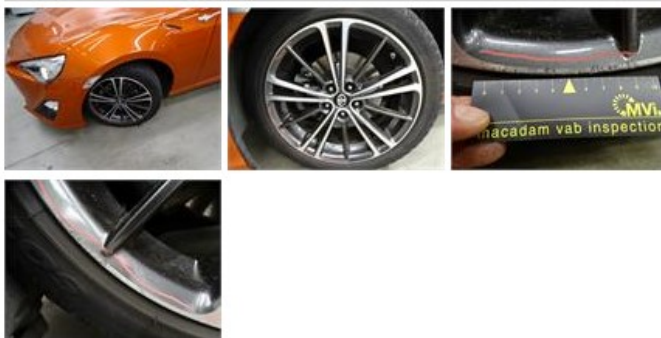
Alloy rim F L polished, Scratch(es), LI - Repair and paint (complete) 95,00
