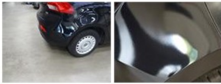
Wing R R, Chemical polution, LI - Repair and paint (complete) 308,20
