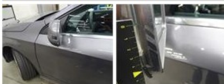
Rearview mirror L complete, Scratch(es), LI - Repair and paint (complete)
