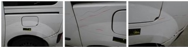
Door F L, Scratch(es), LI - Repair and paint (complete) 318,35
