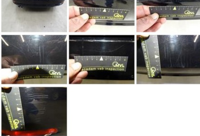
Sill outer L, Deformed / Strained, Le - Replace and paint 712,00
