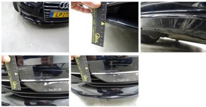
Sill outer R, Scratch(es), LI - Repair and paint (complete) 310,50
