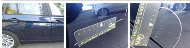
Sill outer R, Scratch(es), LI - Repair and paint (complete) 310,50
