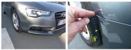
Wing R L, Dent(s) and scratch(es), LI - Repair and paint (complete) 417,84
