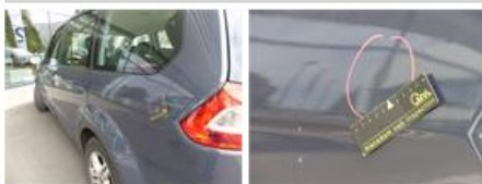
Sill outer R, Scratch(es), LI - Repair and paint (complete) 372,60
