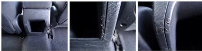
Door R L, Dent(s) and scratch(es), LI - Repair and paint (complete) 318,35
