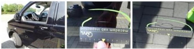
Bumper R, Deformed / Strained, E - Replace 329,40
