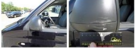
Door F L, Dent(s) and scratch(es), LI - Repair and paint (complete) 238,76
