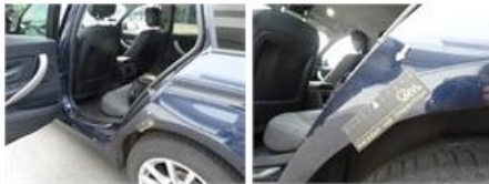
Rocker panel inner R L, Dent(s), LI - Repair and paint (complete) 115,56
