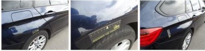
Wing R R, Scratch(es), LI - Repair and paint (complete) 308,20
