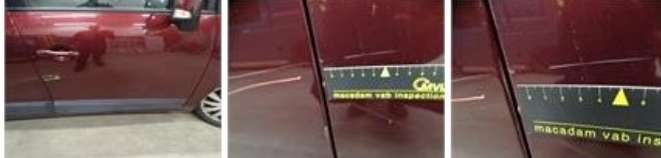
Door R R, Scratch(es), LI - Repair and paint (complete) 318,35
