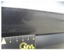
Alloy rim R R polished, Scratch(es), LI - Repair and paint (complete) 95,00
