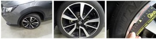
Alloy rim F L polished, Scratch(es), LI - Repair and paint (complete) 95,00
