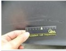
Wing R R, Scratch(es), It - Spot repair 115,56
