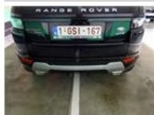
Bumper R, Broken, Le - Replace and paint
