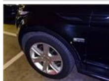
Wing moulding F L, Scratch(es), E - Replace
