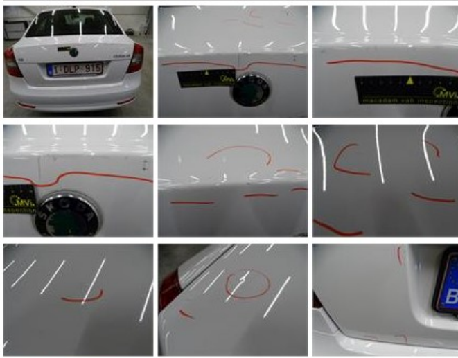
Tailgate, Dent(s) and scratch(es), LI - Repair and paint (complete) 301,68
