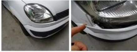
Wing F L, Dent(s) and scratch(es), LI - Repair and paint (complete) 220,18
