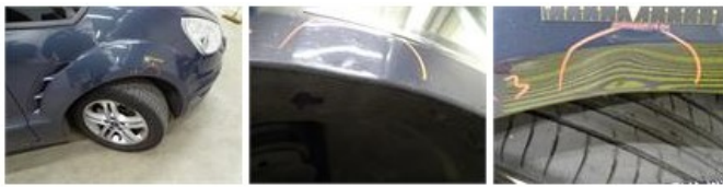
Wing R L, Dent(s) and scratch(es), Le - Replace and paint 1429,81
