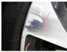
Wing F L, Scratch(es), LI - Repair and paint (complete) 220,18
