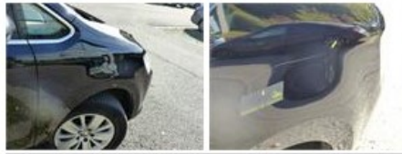
Outer door handle R L, Scratch(es), LI - Repair and paint (complete) 115,56
