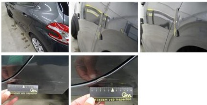
Door panel R L, Scratch(es), Smart repair 110,64
