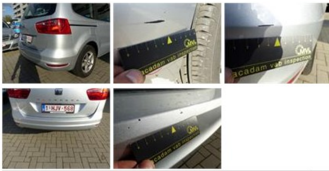
Trunk lid covering R, Scratch(es), Smart repair 110,64
