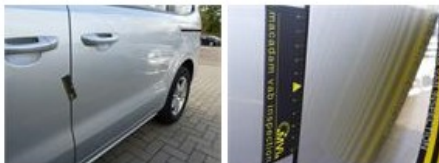
Wing F L, Dent(s), PDR - Paintless dent repair 63,00
