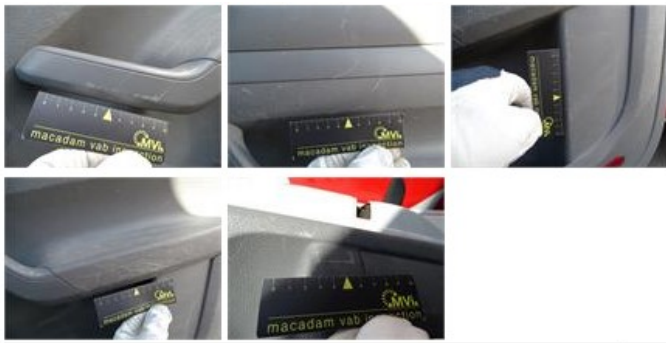
Sliding door R, Dent(s) and scratch(es), LI - Repair and paint (complete) 382,02
