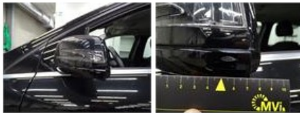
Rearview mirror housing L, Scratch(es), LI - Repair and paint (complete) 115,56
