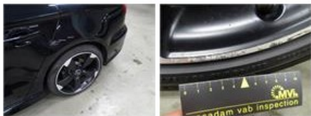
Sill outer L, Scratch(es), It - Spot repair
