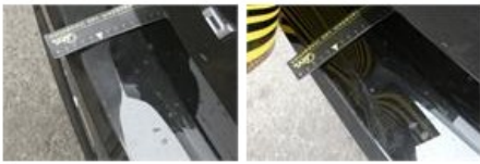
Roof pillar R, Scratch(es), LI - Repair and paint (complete)
