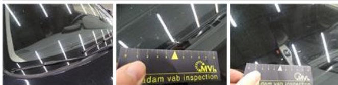
Roof, Dent(s), Acceptable
