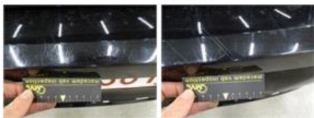
Windscreen, Stone chip(s), Windscreen repair
