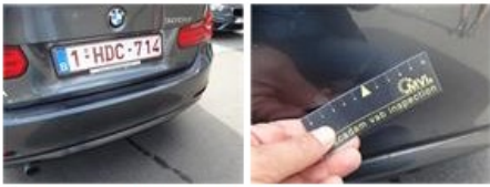
Sill outer L, Scratch(es), It - Spot repair
