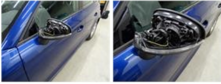
Rearview mirror housing L, Broken, LI - Repair and paint (complete)
