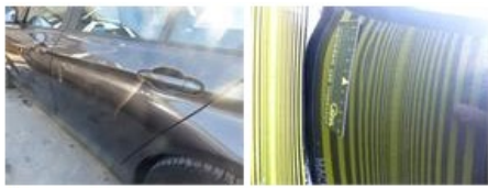
Door panel R R, Scratch(es), Acceptable
