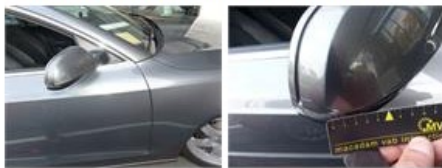
Door F L, Dent(s) and scratch(es), It - Spot repair
