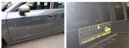
Wing F L, Scratch(es), LI - Repair and paint (complete)
