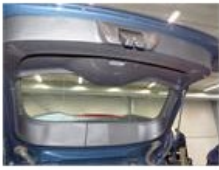
Trunk lid covering R, Scratch(es), E - Replace
