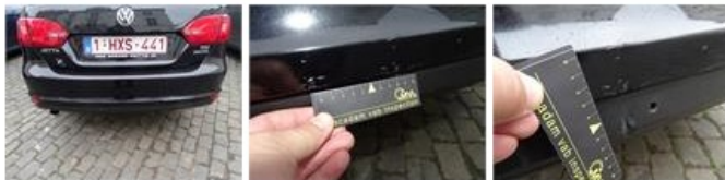
Bumper R, Dent(s) and scratch(es), LI - Repair and paint (complete)
