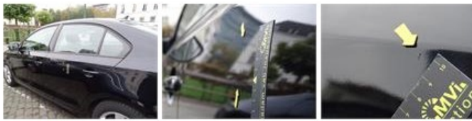
Sill outer L, Dent(s) and scratch(es), LI - Repair and paint (complete)
