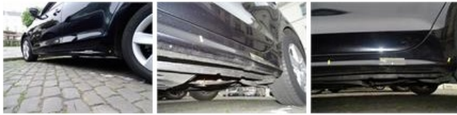
Sill outer L, Dent(s) and scratch(es), LI - Repair and paint (complete)
