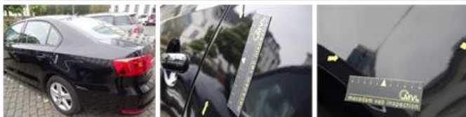
Wing R L, Bad repair, P - Check
