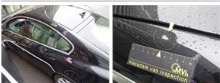
Roof pillar L, Hail damage, PDR - Hail
