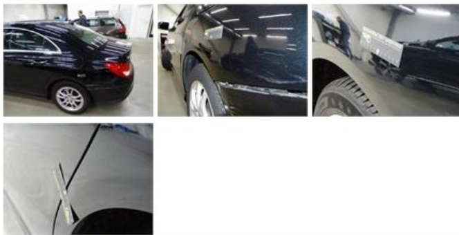
Bonnet, Dent(s), PDR - Paintless dent repair
