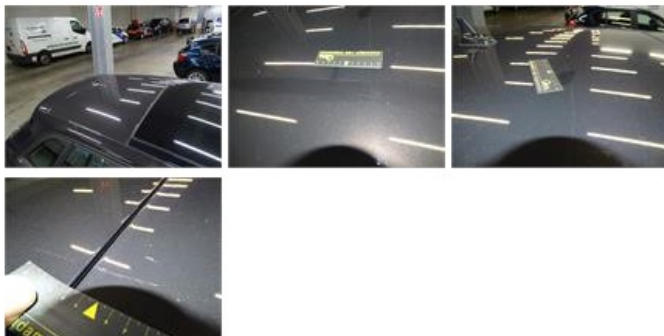
Rearview mirror housing R, Scratch(es), Acceptable
