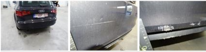
Boot cover, Broken, E - Replace
