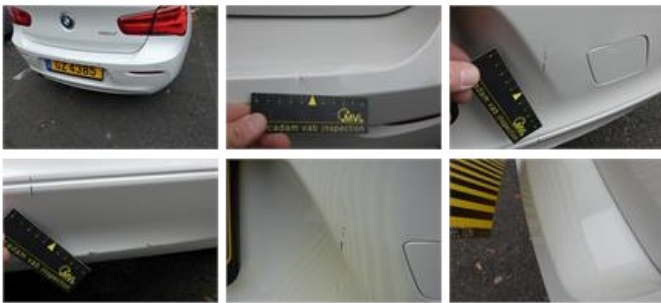
Bumper R, Dent(s) and scratch(es), LI - Repair and paint (complete)
