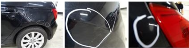
Tailgate, Chemical pollution, LI - Repair and paint (complete)
