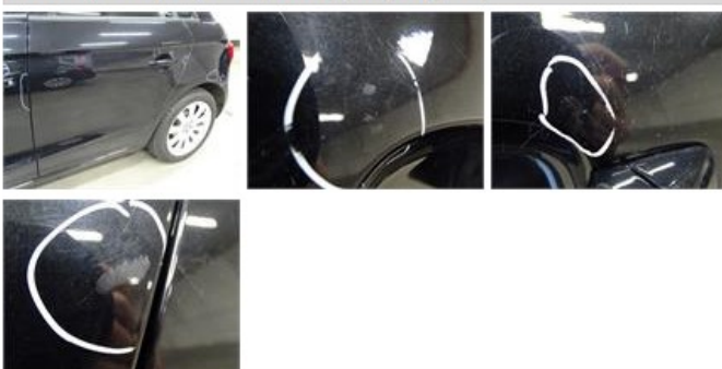
Wing R R, Bad repair, LI - Repair and paint (complete)
