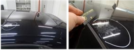
Door F L, Bad repair, LI - Repair and paint (complete)
