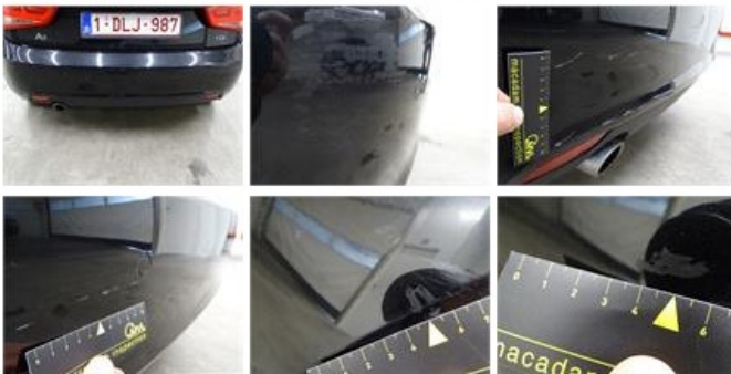
Wing R L, Bad repair, LI - Repair and paint (complete)
