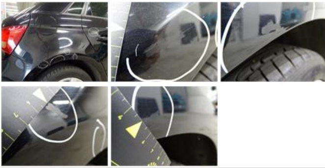
Bumper F, Chemical polution, LI - Repair and paint (complete)
