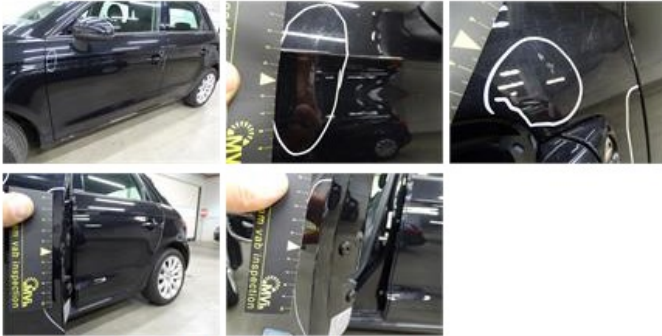
Door R R, Bad repair, LI - Repair and paint (complete)
