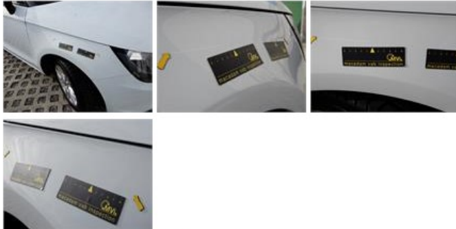
Door R R, Scratch(es), LI - Repair and paint (complete)
