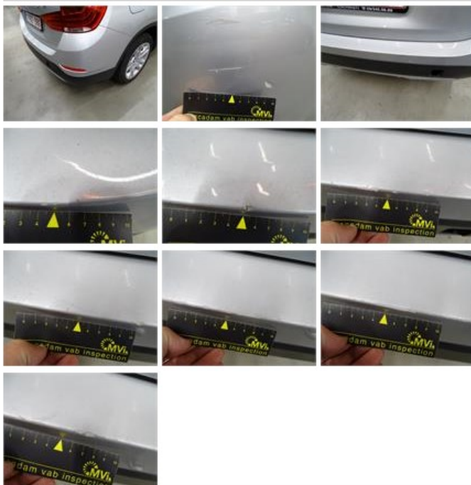
Bumper R, Missing, E - Replace
