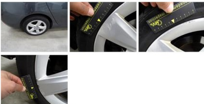
Alloy rim F R, Scratch(es), LI - Repair and paint (complete)
