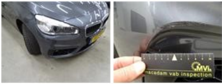
Bumper R, Broken, Le - Replace and paint
