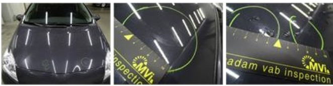
Wing R R, Dent(s), It - Spot repair
