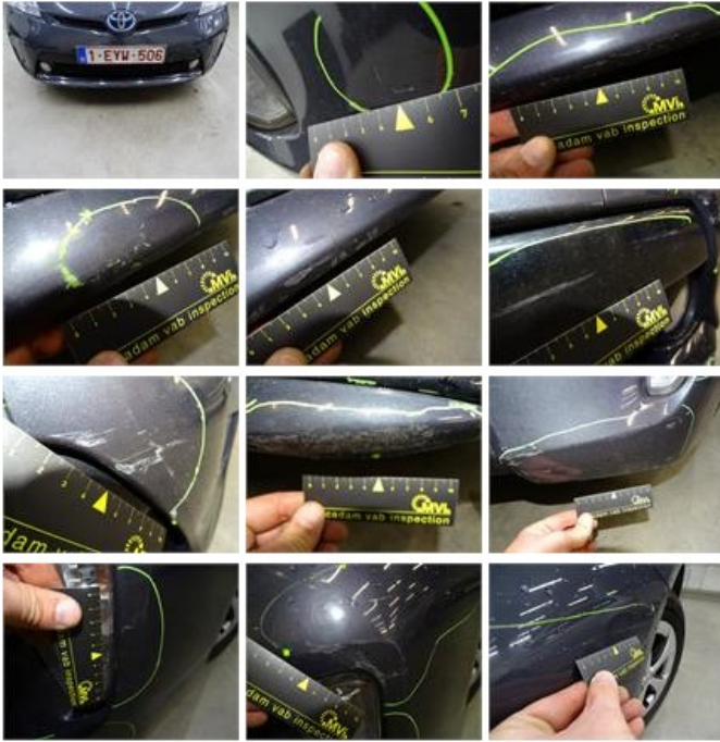
Bumper R, Dent(s) and scratch(es), LI - Repair and paint (complete)
