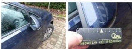
Door R R, Dent(s) and scratch(es), LI - Repair and paint (complete) 318,35
