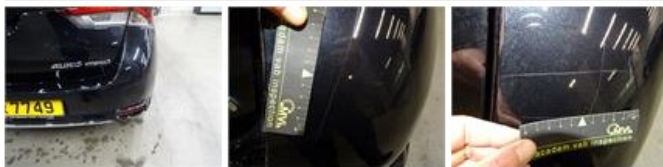
Tailgate, Scratch(es), LI - Repair and paint (complete)
