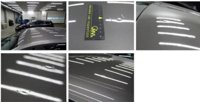
Roof, Hail damage, PDR - Hail
