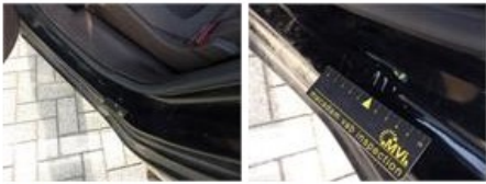
Roof pillar L, Dent(s), Acceptable
