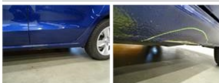
Sill outer L, Dent(s) and scratch(es), It - Spot repair
