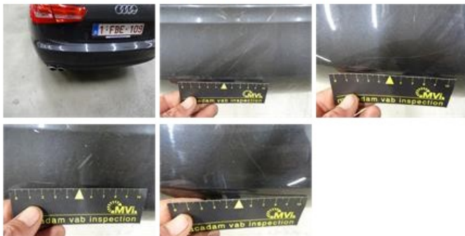
Bumper F, Scratch(es), LI - Repair and paint (complete)
