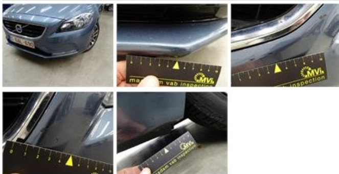
Bumper corner R L, Scratch(es), It - Spot repair
